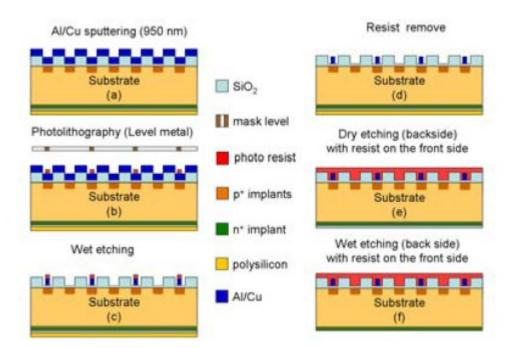
It is important to design the sensor to prevent high field regions. Care has to be taken in the design of metallisation and implants
