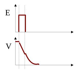
If the potential on the metal is very much above the voltage of the semiconductor the holes are pushed even further away from the semiconductor-oxide interface. Thermally generated electron-holes pairs are separated from each other thus an inversion layer of electrons is built up at the interface. This is called <u>Inversion condition</u>.
