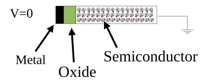
MOS structure (or more general Metal-Insulator-Semiconductor, MIS) is widely used in electronics industry to make gates and in sensor industry to make AC-coupled sensors
