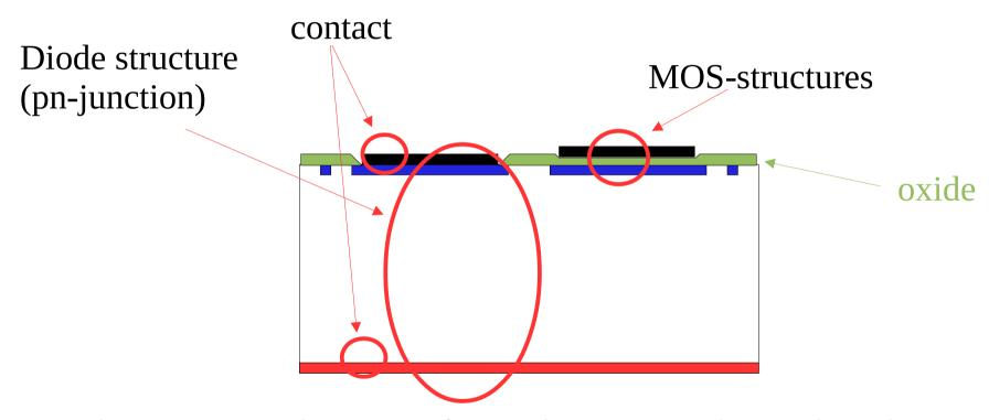
Most important and commonly used structures in semiconductor sensors are
