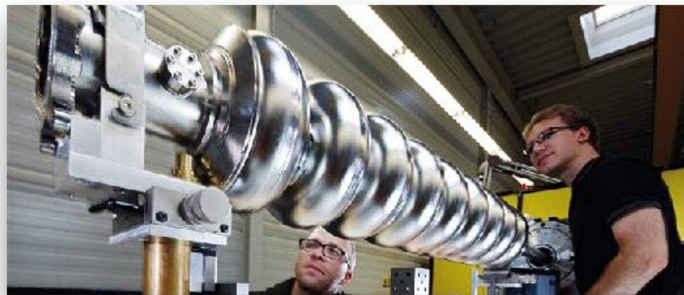
One of the niobium-based 1.3 GHz superconducting RF cavities proposed to be used at the ILC
