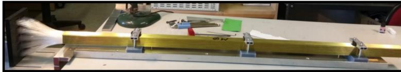
Central tower loaded with fibers
