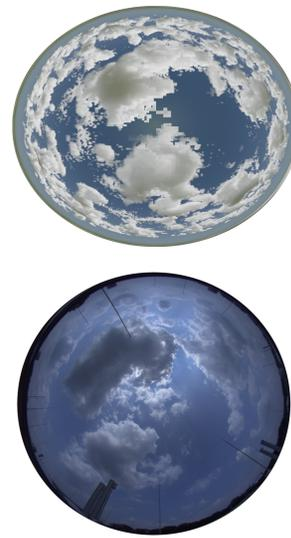
Figure 2: Artificially generated All-Sky Imager emulation of an LES by our path-tracer compared against a real camera image below. Note that the cubic expression reveals the 50 meters horizontal resolution.
