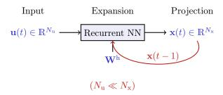
• The recurrent part of the network at any time t is given by:
