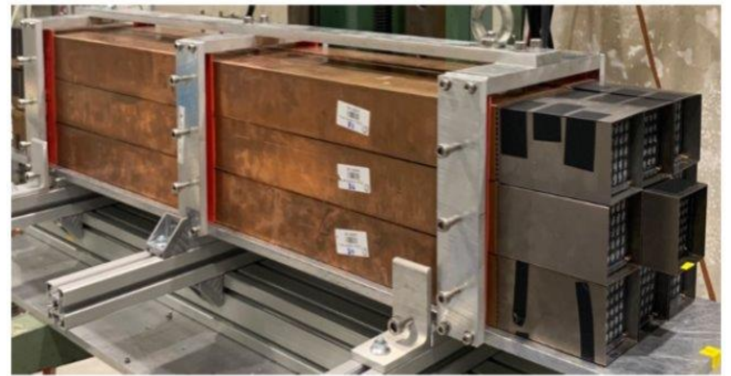
Fig. 1. FoCal-H Prototype 2. Image from a testbeam event September 2023.
