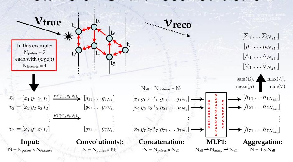
The input features of a node are combined with that of N (=2) nearby nodes through an NN (MLP0) function, yielding an (abstract) vector for each node. This can be repeated (not shown). All the features are then combined (concatenated) into long vectors, which are again put through an NN (MLP1) function with a large hidden layer. The outputs are aggregated in four ways: Min, Max, Sum & Mean, breaking the variation with number of nodes.
