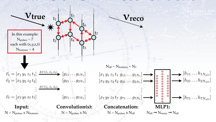
The input features of a node are combined with that of N (=2) nearby nodes through an NN (MLP0) function, yielding an (abstract) vector for each node. This can be repeated (not shown). All the features are then combined (concatenated) into long vectors, which are again put through an NN (MLP1) function with a large hidden layer.
