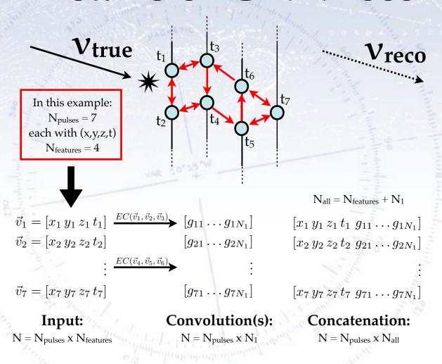
The input features of a node are combined with that of N (=2) nearby nodes through an NN (MLP0) function, yielding an (abstract) vector for each node. This can be repeated (not shown). All the features are then combined (concatenated) into long vectors,
