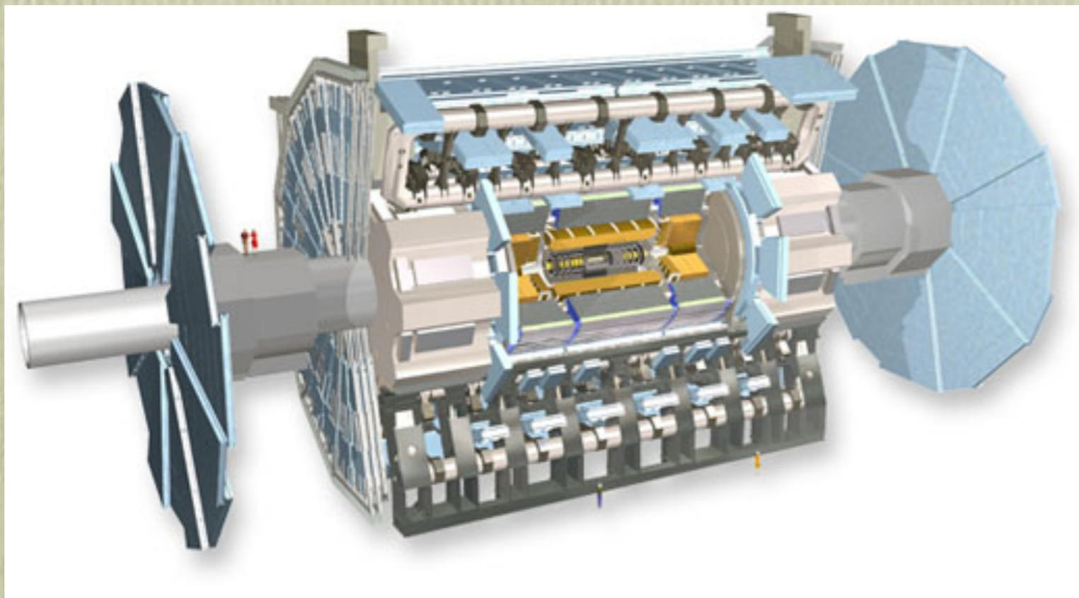
Complete hadronic and electromagnetic calorimeter coverage within  $|\eta| < 4.9$
