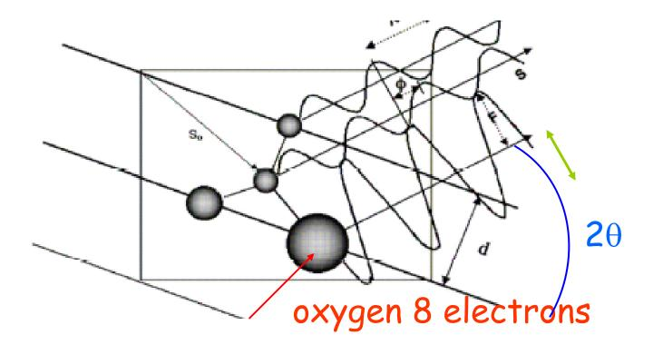
In each reciprocal lattice point we measure a reflection with a given intensity The measured intensity  $I(\underline{H})$
