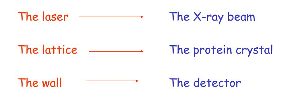
The experiment is successful because the wavelength of the X-rays is comparable with the lattice dimensions in a crystal
