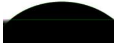
Gold Uncoated Contact Angle = 50^\circ
