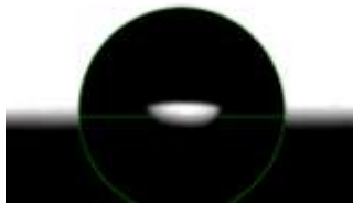
Gold Coated w/PTFE Contact Angle = 93^\circ
