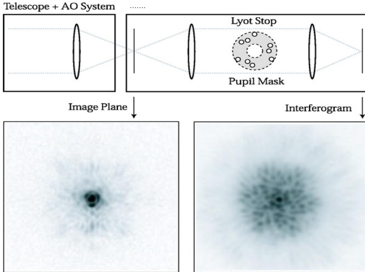
**Nonredundant Mask Interferometry (NRM):** Place an aperture mask in the pupil plane, turning the single mirror into a sparse array. Fourier analysis techniques (i.e. closure phases) filter almost all remaining noise from turbulence and AO errors. (It's called SAM on the VLT.)
