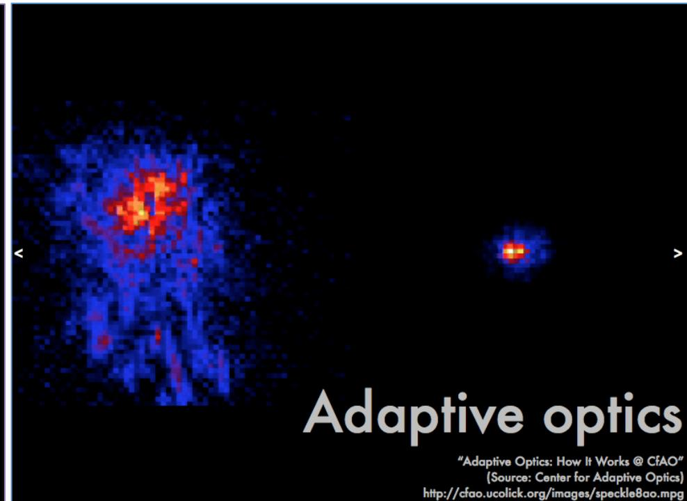
Correct the turbulence introduced by the atmosphere, and hence concentrate the light of the primary star away from the planet.
