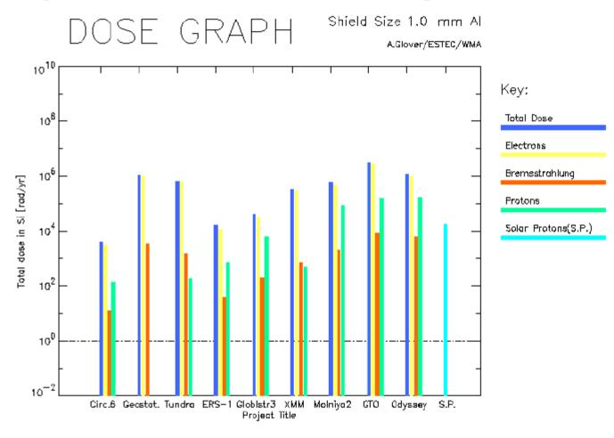
Solar events can produce peak flux (at earth) >  $10^6$  protons/cm<sup>2</sup>/s (>10 MeV) Yearly dose around 1 kGy (100 krad)
