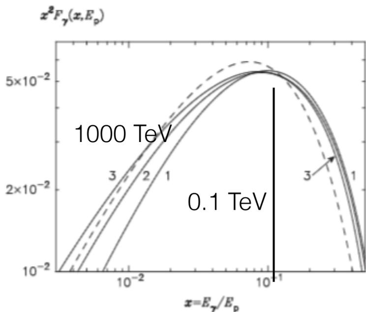
Figure 7: Energy spectra of gamma-rays described by Eq.(58) for three energies of incident protons: 0.1 TeV (curve 1), 100 TeV (curve 2) and 1000 TeV (curve 3). The dashed curve corresponds to the Hillas parameterization of the spectra obtained for proton energies of several tens of TeV.
