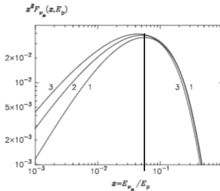
Figure 9: Energy spectra of all muonic neutrinos described by Eq.(62) and (66) for three energies of incident protons: 0.1 TeV (curve 1), 100 TeV (curve 2) and 1000 TeV (curve 3).
