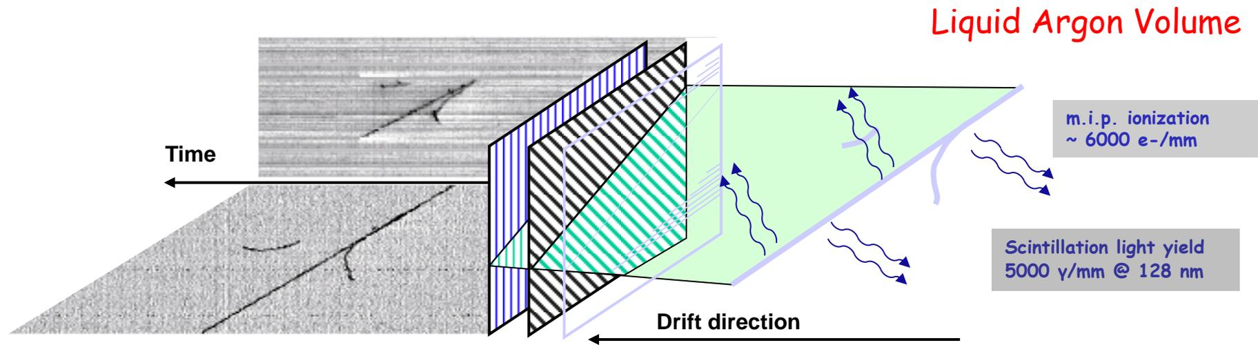
Electrons from ionizing track are drifted in LAr by  $E_{\text{drift}}$ . They traverse two transparent wire arrays oriented in different directions where induction signals are recorded. Finally electron charge is collected by collection plane.
